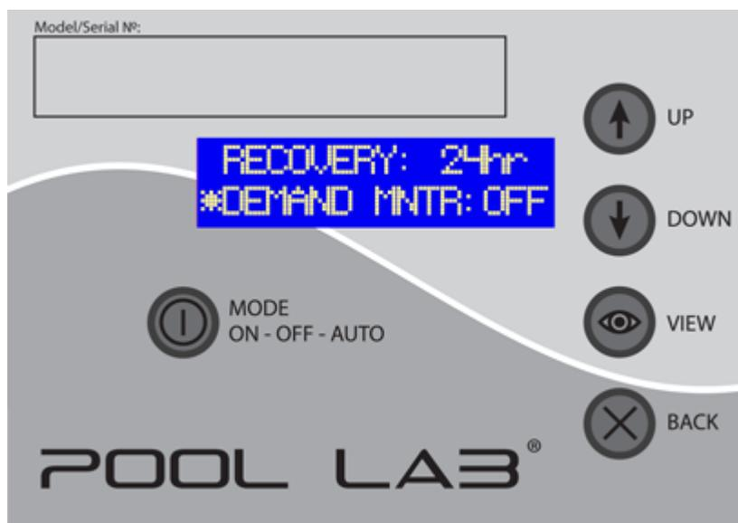
5. Press **VIEW** button and OFF will start flashing. Use **UP** or **DOWN** button to adjust to ON, then press **VIEW** button to set.
