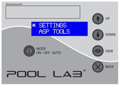
2. Use the **DOWN** button to move the asterisk to **SYSTEM CONFIG:**
