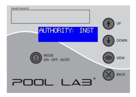
6. Press **VIEW** to set the Authority Level to **INST**, then use the **BACK** button to return to the main menu and adjust settings as required.
