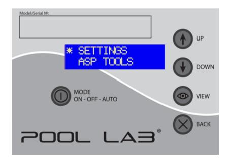
3. Ensure asterisk is next to SETTINGS as per the image above. Press **VIEW** button to enter targets menu:
