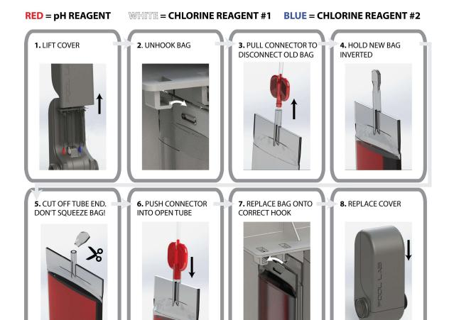
NOTE: After installing new reagent bags, prime the reagent lines by either:
