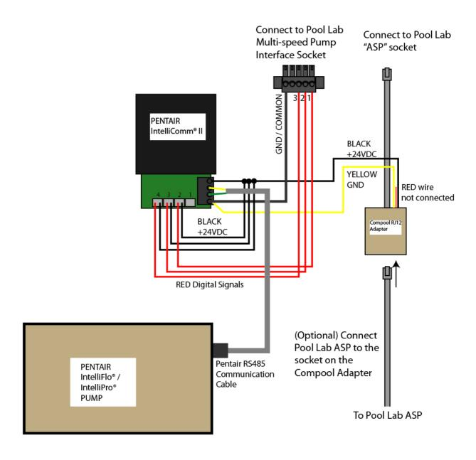
If you have a Pool Lab ASP, you will now need to connect this via the Compool Adapter. Ensure the IntelliComm II and the Compool adapter are protected from weather.
