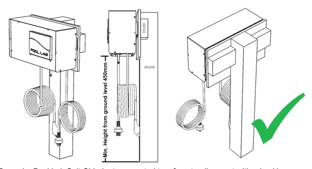
Example: Pool Lab Salt Chlorinator mounted to a freestanding post with a backing board. Ensure the post is secure and all materials used are suitably weatherproofed. The bottom of the unit must be mounted a minimum of 450mm from ground level.
